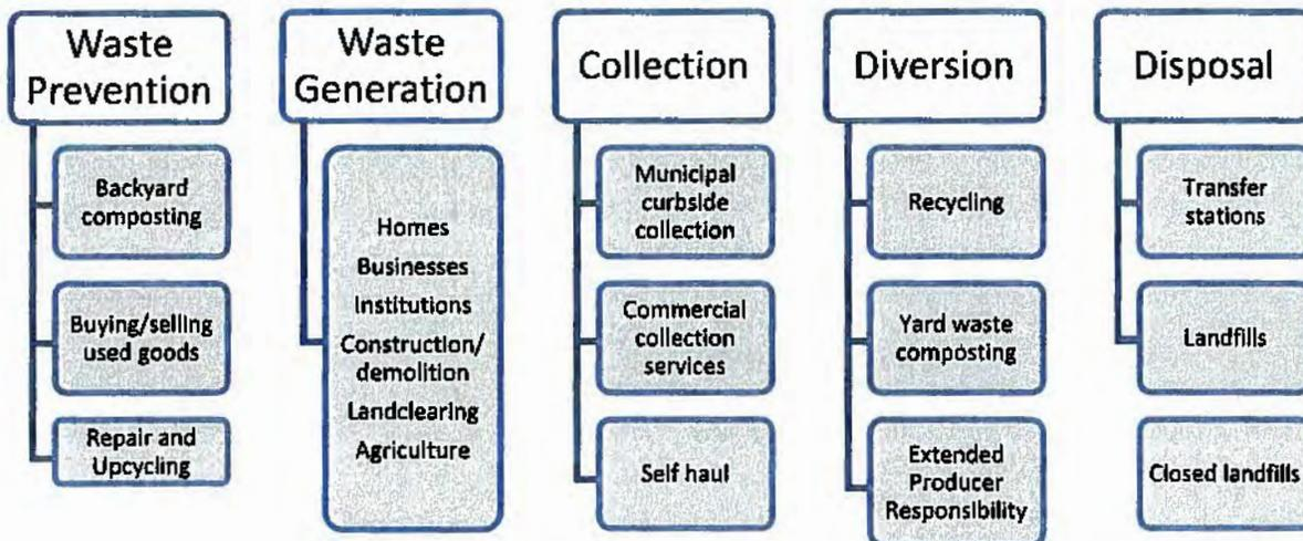
**Figure 3-1: Components of the Waste Management System**
