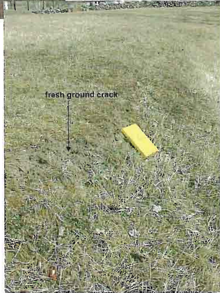
Photo 24: Trace of fresh ground cracking, looking south between 195 and 265 Lower Viewmount Road.
