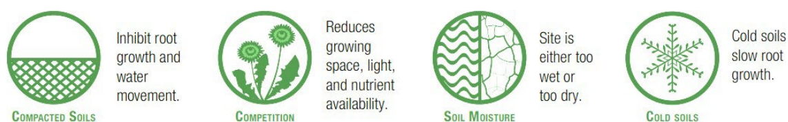
Figure 3.1-1. Common Reclamation Filters (adapted from FLNRO 2021)
