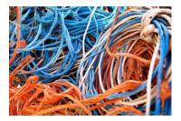
**Bale Wrap** – Bale wrap is made from linear low-density polyethylene (LLDPE) and is used, often in multiple layers, to contain bales after harvest.
