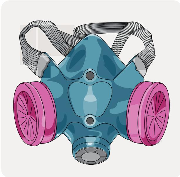
Workers can use half-facepiece, dual-cartridge respirators with P100 (HEPA) filters in asbestos concentrations up to 1 fibre per millilitre.
